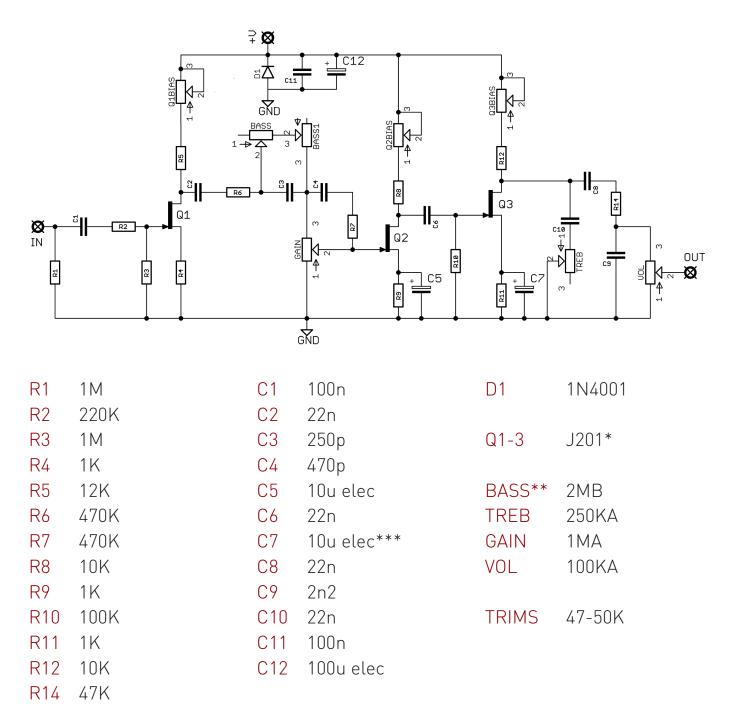
\*Pads are included for through-hole J201 or their SMT equivalent MMBFJ201 which will be easier to source (though harder to solder)
