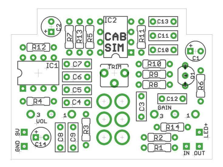
Pots can be mounted in position using header pins or snipped leg components, or just use wire as normal.
