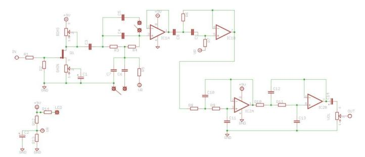
Parts listed in black are for the full build, including the Marshall Notch Depth switch. To build the circuit stock, see values in BLUE for C5-7 and omit the DPDT switch.
