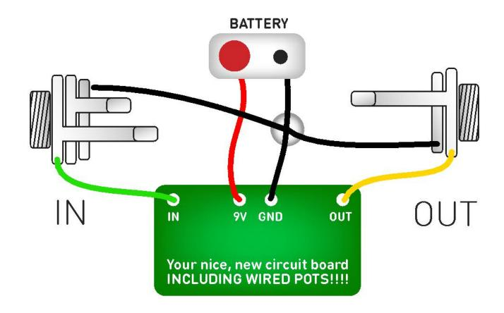
Once you've finished the circuit it makes sense to test is before starting on the switch and LED wiring. It'll cut down troubleshooting time in the long run. If the circuit works at this stage, but it doesn't once you wire up the switch - guess what? You've probably made a mistake with the switch.
