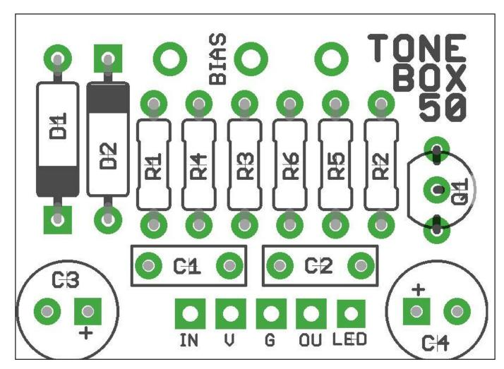
The power and signal pads on the PCB conform to the FuzzDog Direct Connection format, so can be paired with the appropriate daughterboard for quick and easy offboard wiring.
