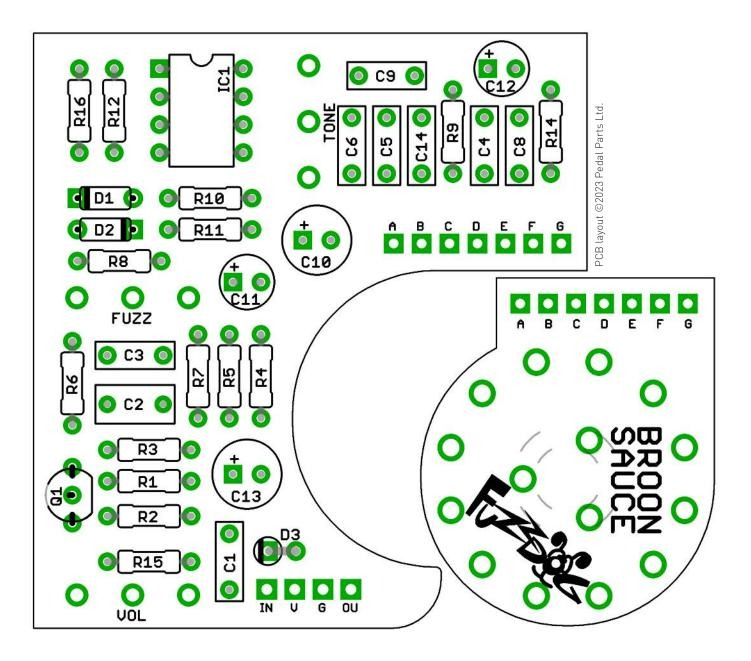
As you can see on the cover image, the rotary switch is mounted on a separate daughterboard. This has been designed to mount with standard header pins (7-way).
