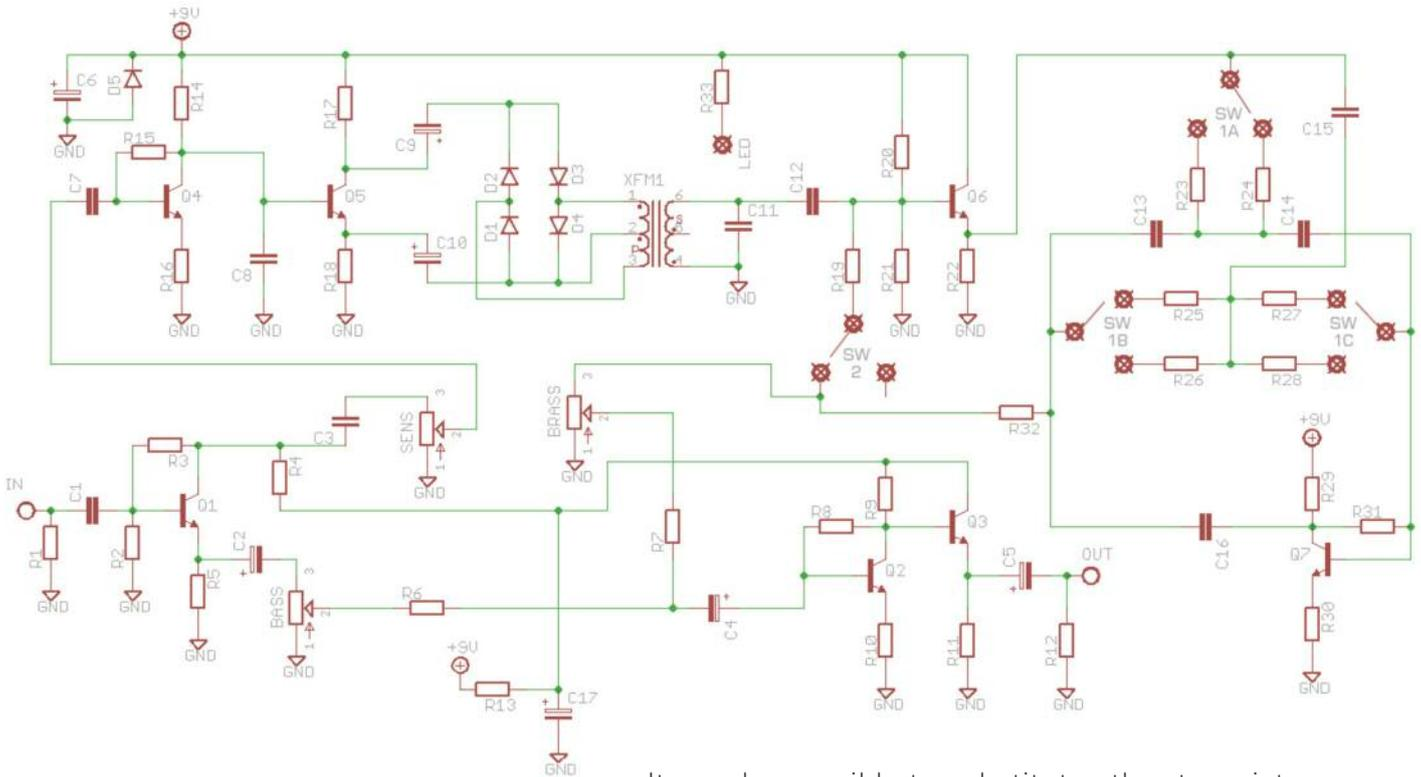
It may be possible to substitute other transistors or transformer. Please don't ask for advice on this as we haven't tested any others, though 2N3391 will work fine for Q1-6.
