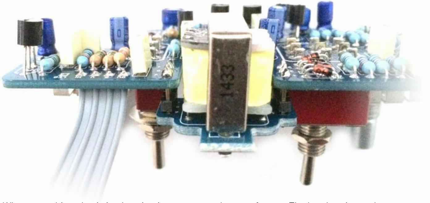
When everything else is in place its time to mount the transformer. The header pins and transformer mount it on the same side of the board as the screenprint showing the transformer and the numbers 1-6.
