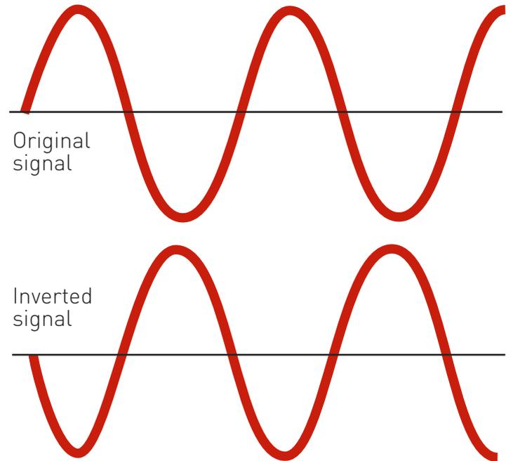
This is a consideration when adding a blender to a circuit. If the end result signal of that circuit is inverted, then blending it with your original signal will result in cancellation, which means volume drop.
