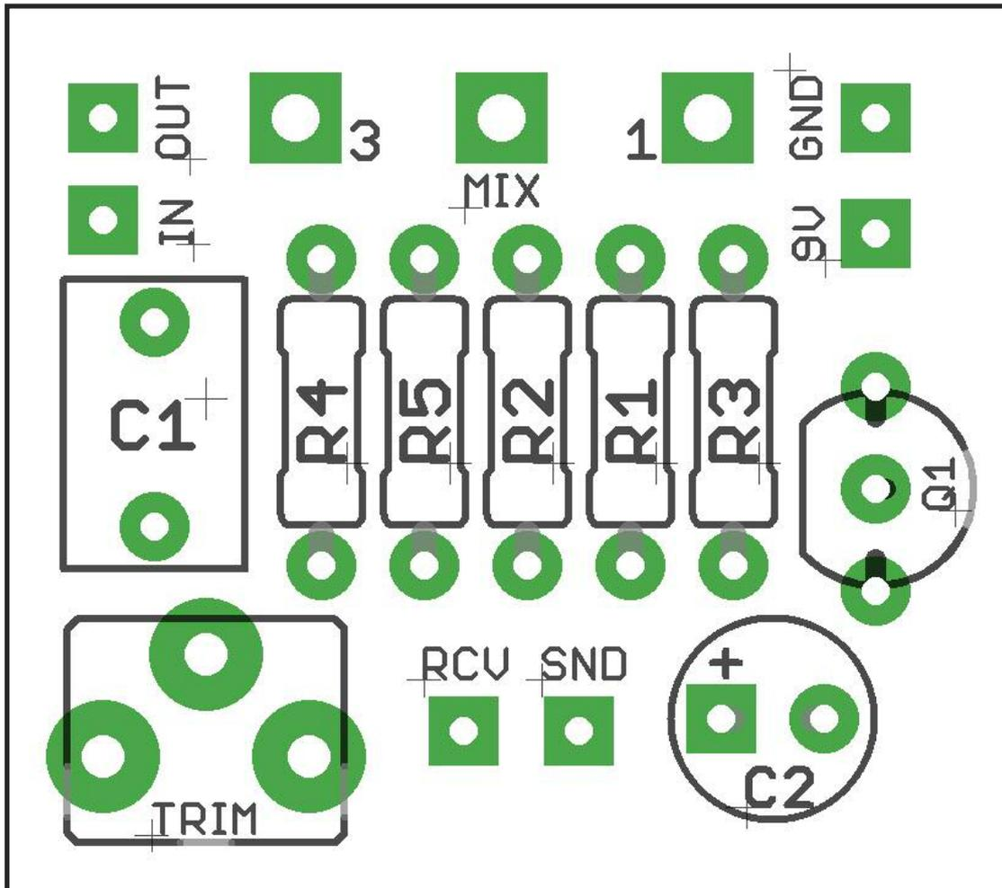
The PCB is designed to have the mix pot mounted directly. You can use wire if you like - simply connect the board pads to the corresponding pins on the pot.
