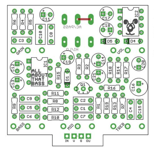
The power and signal pads on the PCB conform to the FuzzDog Direct Connection format, so can be paired with the appropriate daughterboard for quick and easy offboard wiring. Check the separate daughterboard document for details.
