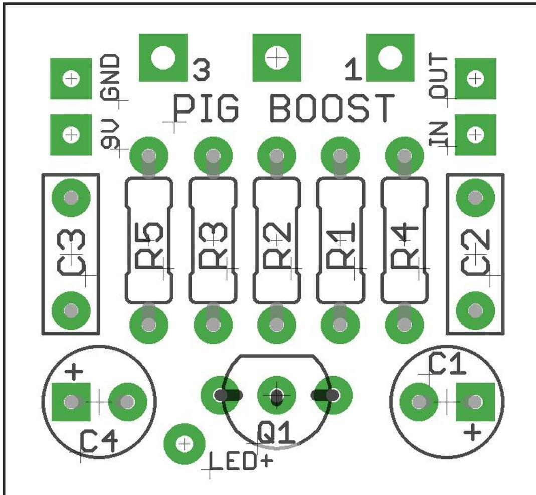
The PCB is designed to have the boost pot mounted directly. You can use wire if you like - simply connect the board pads to the corresponding pins on the pot.
