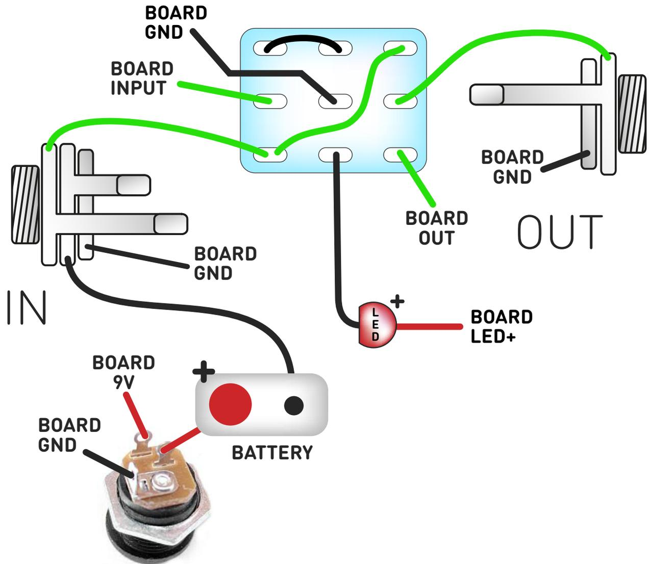
The Board GND connections don't all have to directly attach to the board. You can run a couple of wires from the DC connector, one to the board, another to the IN jack, then daisy chain that over to the OUT jack.
