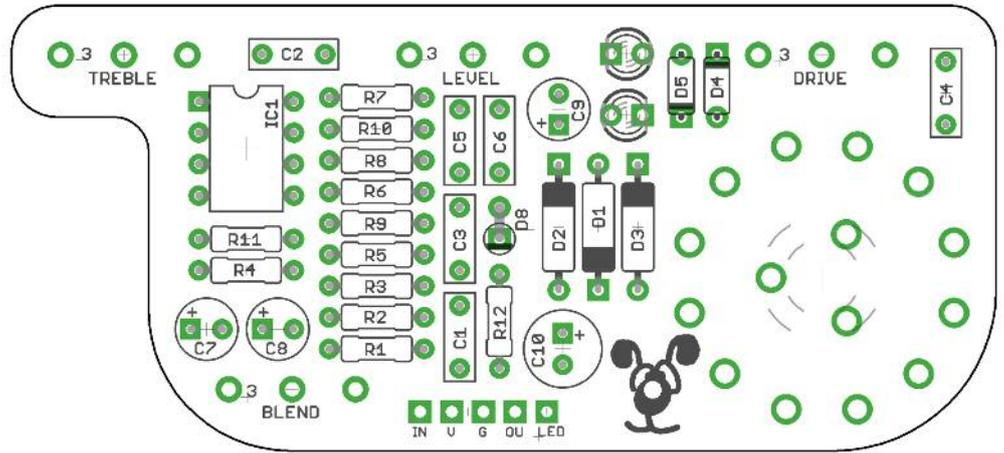
The power and signal pads on the PCB conform to the FuzzDog Direct Connection format, so can be paired with the appropriate daughterboard for quick and easy offboard wiring.
