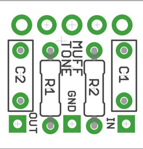
There are two sets of pads for the pot to enable the use of 16mm or 9mm in either horizontal or vertical pin format.
