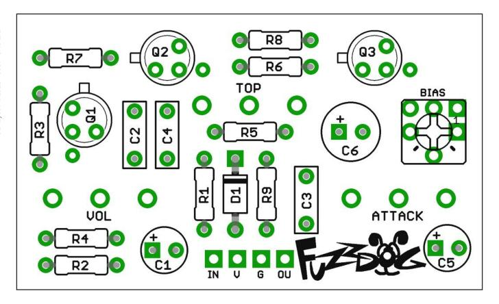
The power and signal pads on the PCB conform to the FuzzDog Direct Connection format, so can be paired with the appropriate daughterboard for quick and easy offboard wiring. Check the separate daughterboard document for details.
