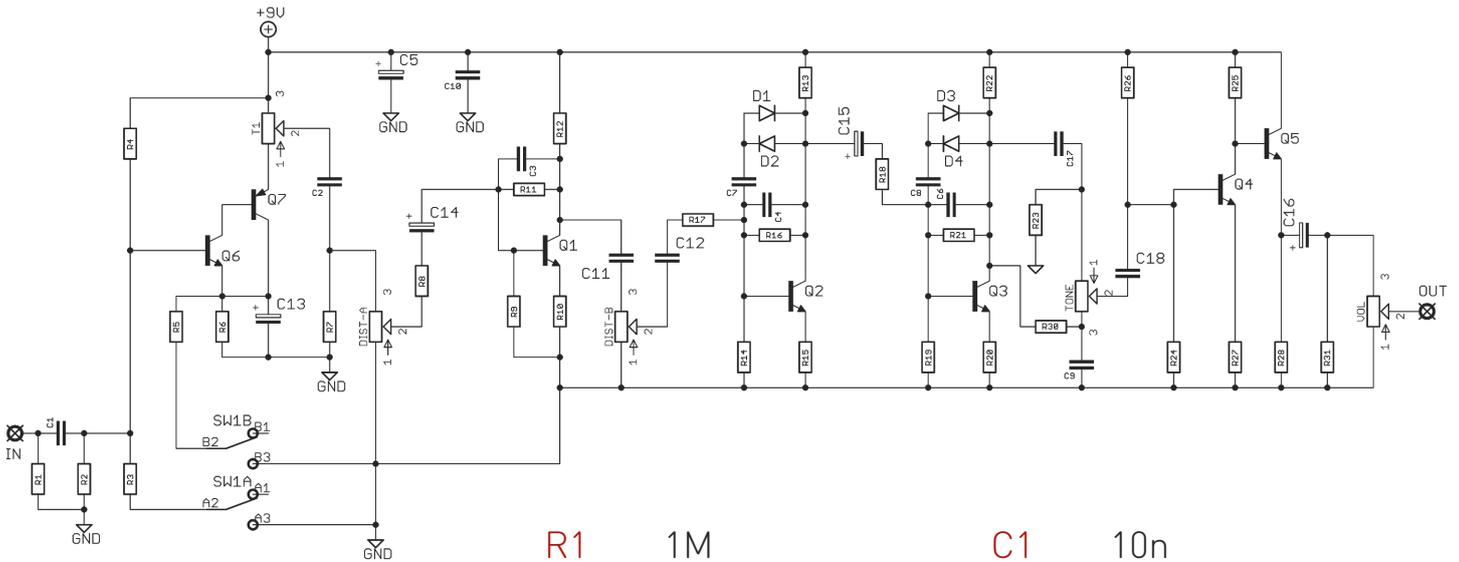
\*The original circuit uses C2240, but you could try other BJT. The circuit is basically a Big Muff Pi. C2240 have a non-standard pin-out so there are extra pads on the PCB to accomodate those and standard CBE cans. See later in this document for more info on that.
