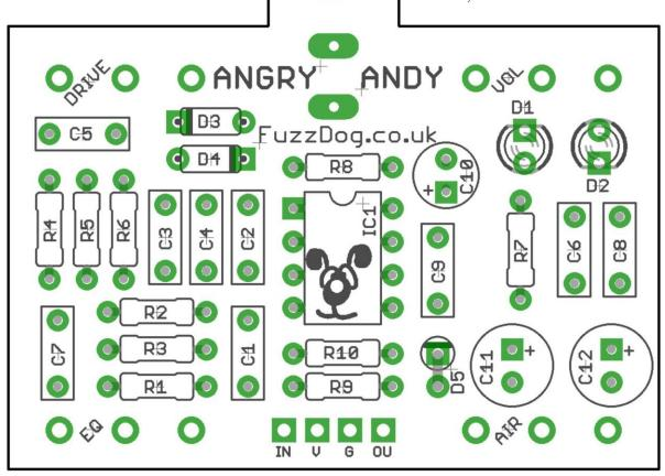
The power and signal pads on the PCB conform to the FuzzDog Direct Connection format, so can be paired with the appropriate daughterboard for quick and easy offboard wiring. Check the separate daughterboard document for details.
