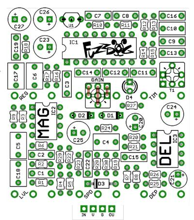
The power and signal pads on the PCB conform to the FuzzDog Direct Connection format, so can be paired with the appropriate daughterboard for quick and easy offboard wiring. Check the separate daughterboard document for details.
