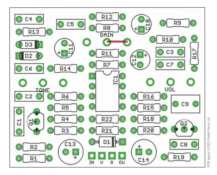
To omit the GAIN control simply add a jumper as shown above in red in place of the pot.
