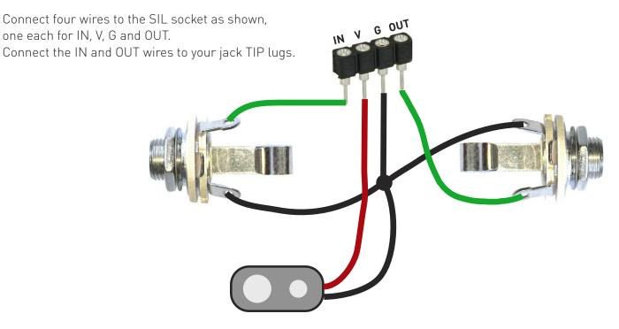
Now for your power. ALL the ground connections have to join together. Twist together a bare end of all the GND wires - one from the SIL socket, one from each jack, and your battery negative lead. Solder that clump all together. Connect your battery positive lead to the V lead from the socket. You now have a Direct Connect tester.
