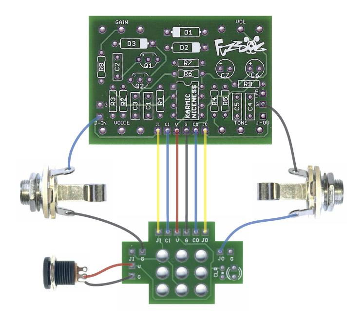
In the case above the Enlightned MkII PCB has six corresponding pads with the daughterboard, including Jack In and Jack Out. It can be connected with 6 wires or ribbon cable. You then have the choice of taking the Jack Signal and GND connections from either board which can make your wiring shorter and neater.
