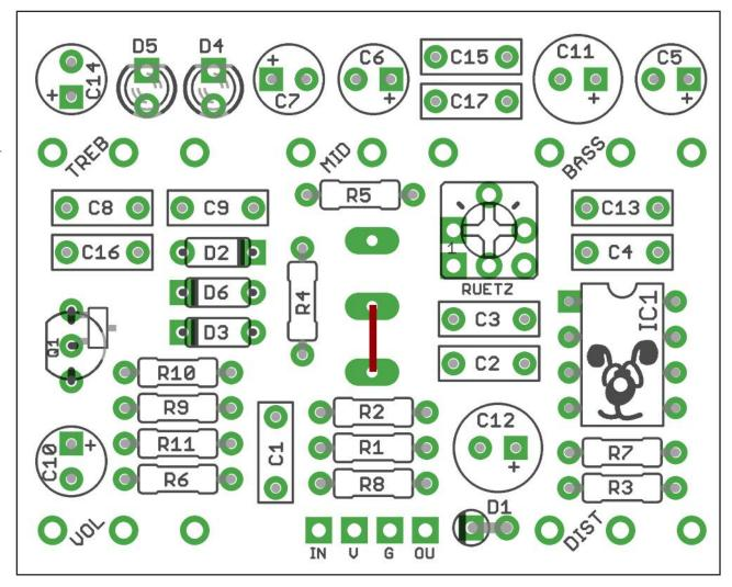
The power and signal pads on the PCB conform to the FuzzDog Direct Connection format, so can be paired with the appropriate daughterboard for quick and easy offboard wiring. Check the separate daughterboard document for details.
